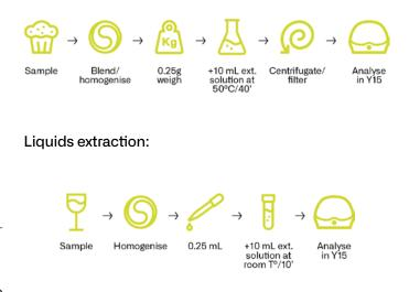
Once extracted, the liquid sample is placed in the autoanalyser, giving direct results in ppm within 10 minutes for the first sample (with a capacity of up to 75 tests per hour).
